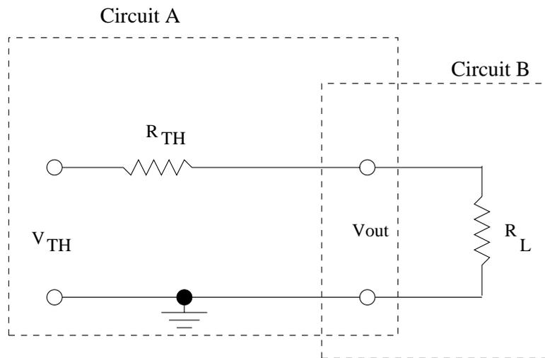
Figure 6: Two interacting circuits.
