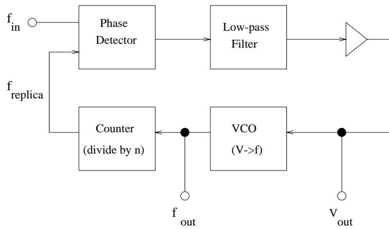
Figure 45: PLL schematic.  $V_{out}$  provides the FM signal.
