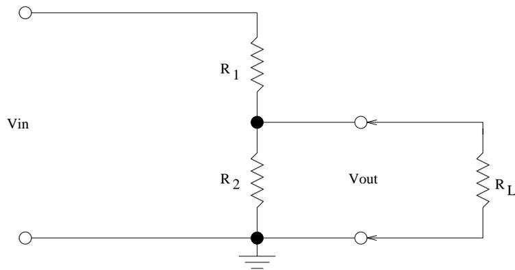
Figure 4: Adding a “load” resistor  $R_L$ .
