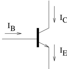
Figure 17: Transistor currents.
