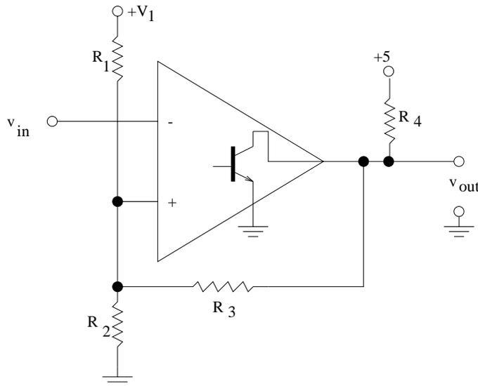
Figure 39: Schmitt trigger.
