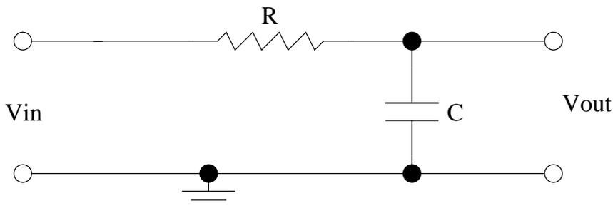
Figure 11: A low-pass filter.
