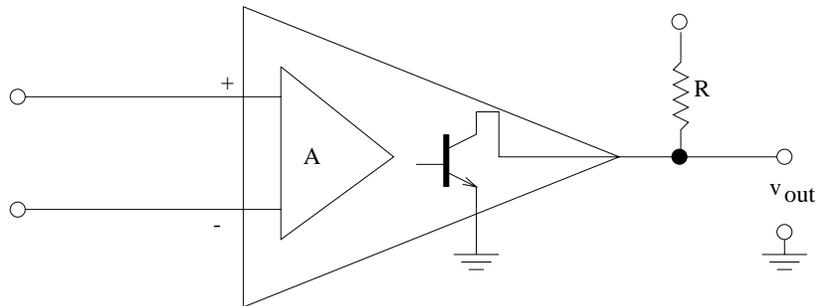
Figure 38: Comparator model.
